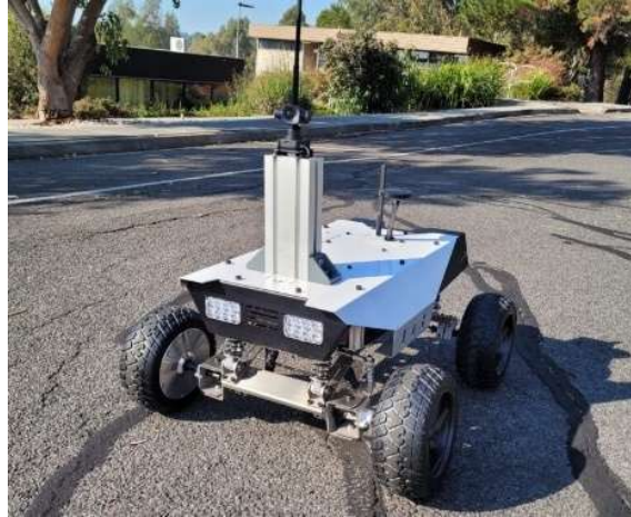
Figure 1: The EywaGuard robotic platform featuring a gimbaled camera, GPS, independent suspension, and rugged 4-wheel chassis.
